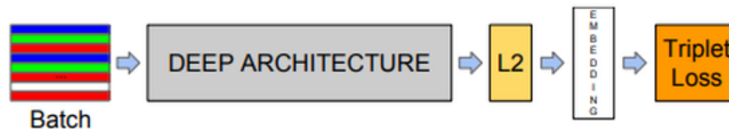
Figure 2. Model structure. Our network consists of a batch input layer and a deep CNN followed by L_2 normalization, which results in the face embedding. This is followed by the triplet loss during training.
